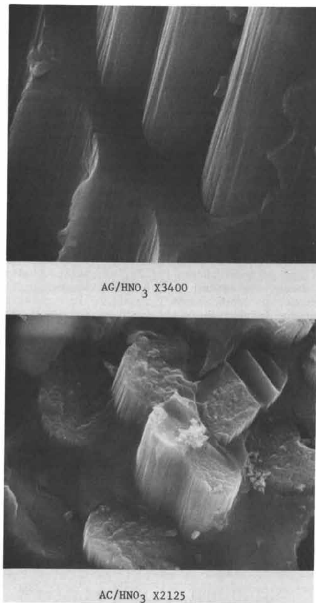
Figure 3. Fracture of the composite after acidic etching of the fibers
