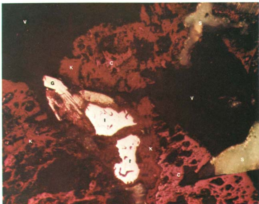
Plate XIV. Inland steel test—S. Chicago, Ind. Formcoke reductant recovered from the ladle.
