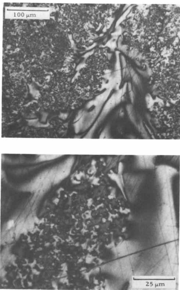
Figure 10. The microstructure of a needle coke particle, viewed perpendicular to the length of the particle. Region A of Figure 9. Crossed polarizers.
