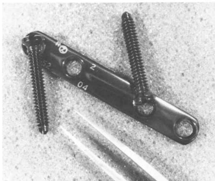
Figure 18. A bone plate and screws coated with an adherent, thin layer of impermeable isotropic carbon
